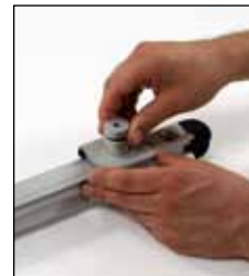
6 Replace the plunger or tamper proof stop. Ensure that the tamper proof stop is secured with a torque setting of 15kN or that the pin on the plunger stop is engaged with the hole in the rail.
