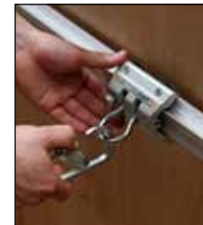
7 Attach your karabiner and lanyard to the rail carriage via the carriage shackle. Ensure the karabiner is locked and secure.
