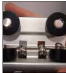
1 Inspect the rail carriage ensuring that the wheels are secure and the security clips are in place.
