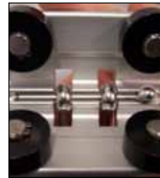
2 Ensure that the shackle pin is present and undamaged.
