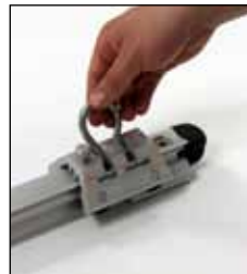
5 Slide the carriage on to rail ensuring the wheels are free to move.
