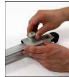
3 If the system is installed with a plunger stop, pull up the head of the stop and slide it from the end of the rail.
